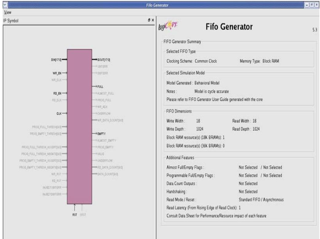
The screenshot displays the 'Fifo Generator' configuration summary screen. The left pane shows the IP Symbol block diagram with various input and output signals. The right pane shows the 'Fifo Generator' configuration summary.
