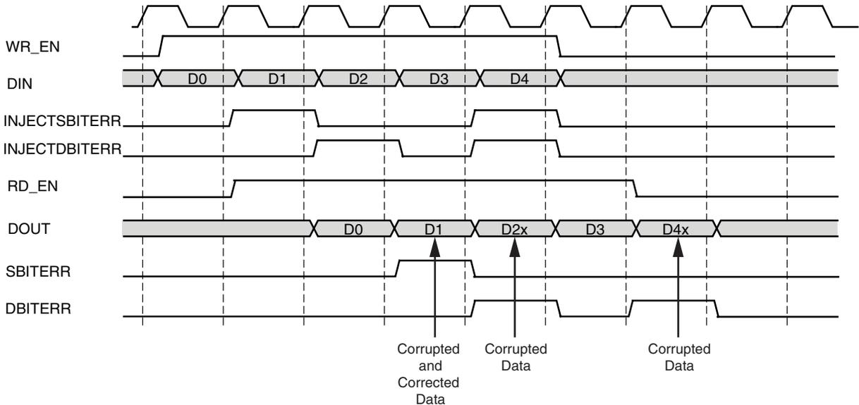
Figure 4-25: Error Injection and Correction in Virtex-6 FPGA
