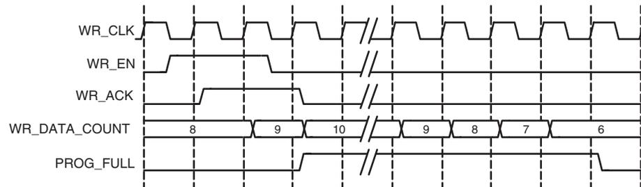
Figure 4-13: Programmable Full with Assert and Negate Thresholds: Assert Set to 10 and Negate Set to 7
