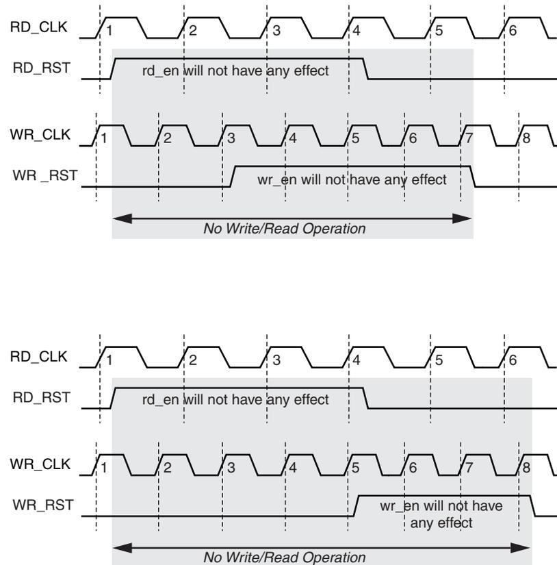
Figure 4-34: Synchronous Reset: FIFO with Independent Clock - RD\_RST then WR\_RST
