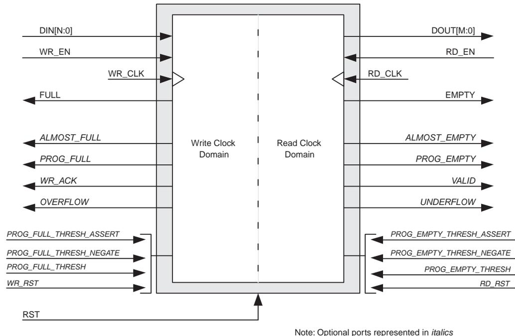
Figure 2-1: FIFO with Independent Clocks: Interface Signals
