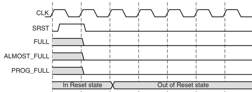
Figure 4-32: Synchronous Reset: FIFO with a Common Clock
